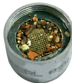
Rust particles in a tap sieve indicate corrosion is present
